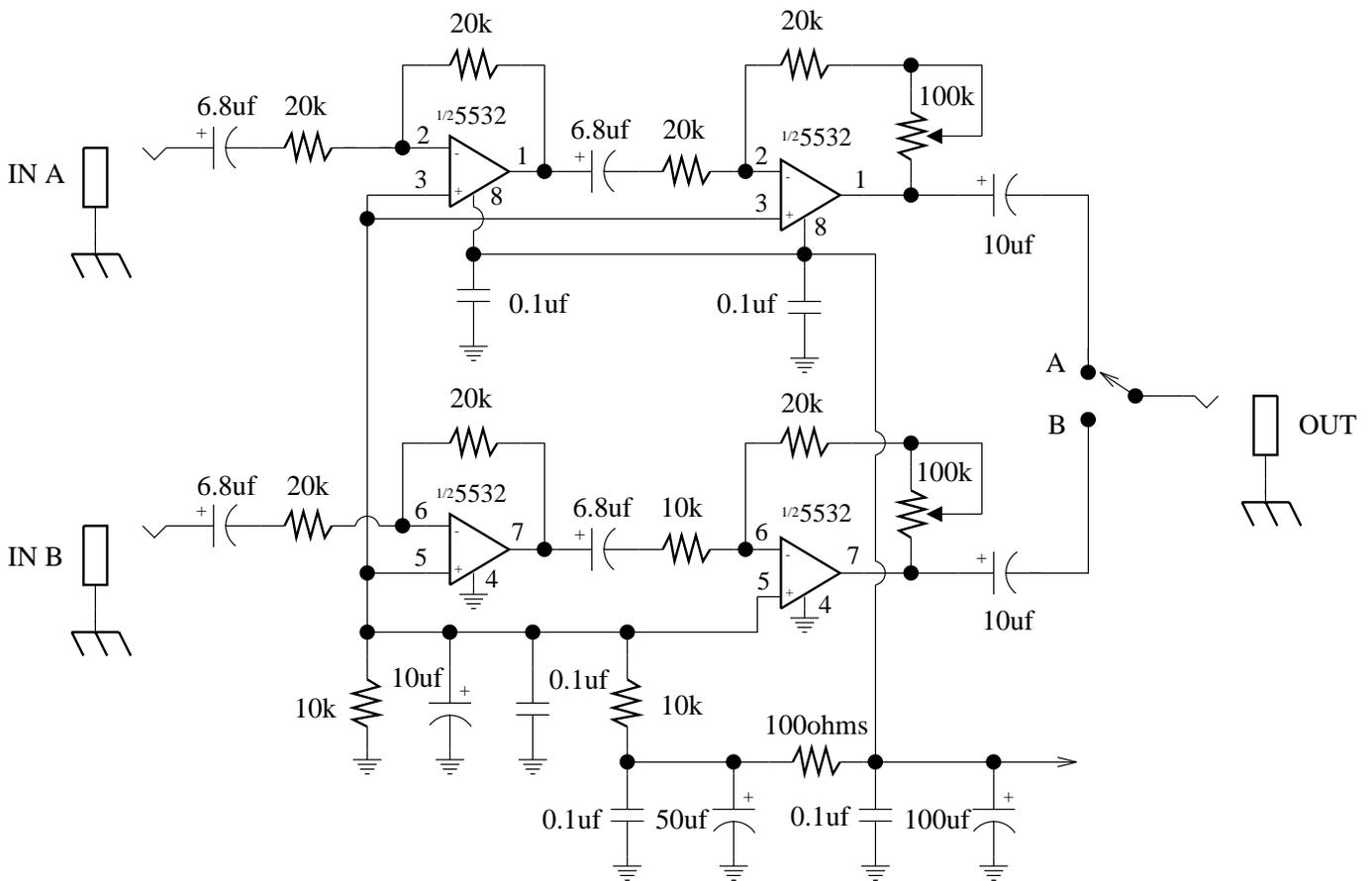
This low noise preamp & a/b box was originally designed for switching between different harmonica mics.
