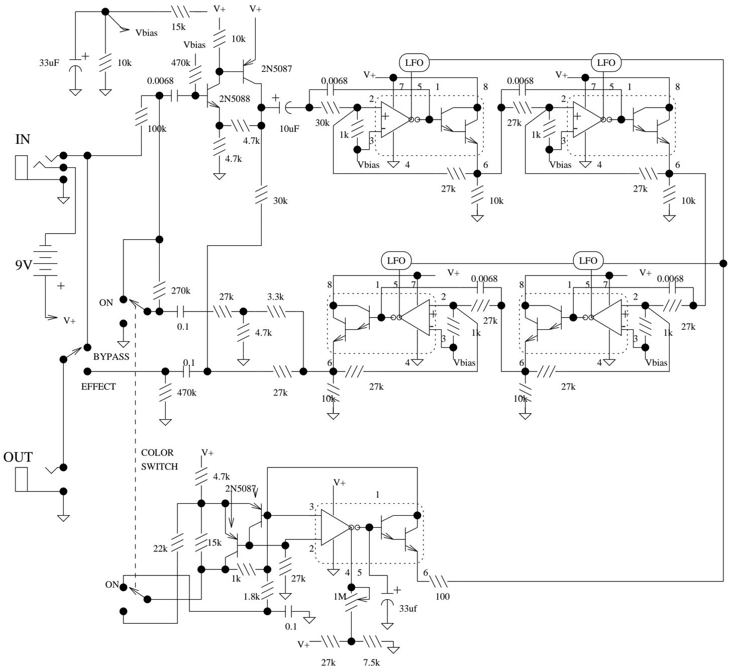
The Small Stone is somewhat unique in using Operational Transconductance Amplifiers (OTA's) for phase shift stages instead of opamps with variable resistors. All of the IC's are house marked EH1048, but can be replaced with CA3094 which is a combination of an OTA equal to the CA3080 and a darlington emitter follower. Later Small Stones used slightly different circuits, but all used the OTA.
