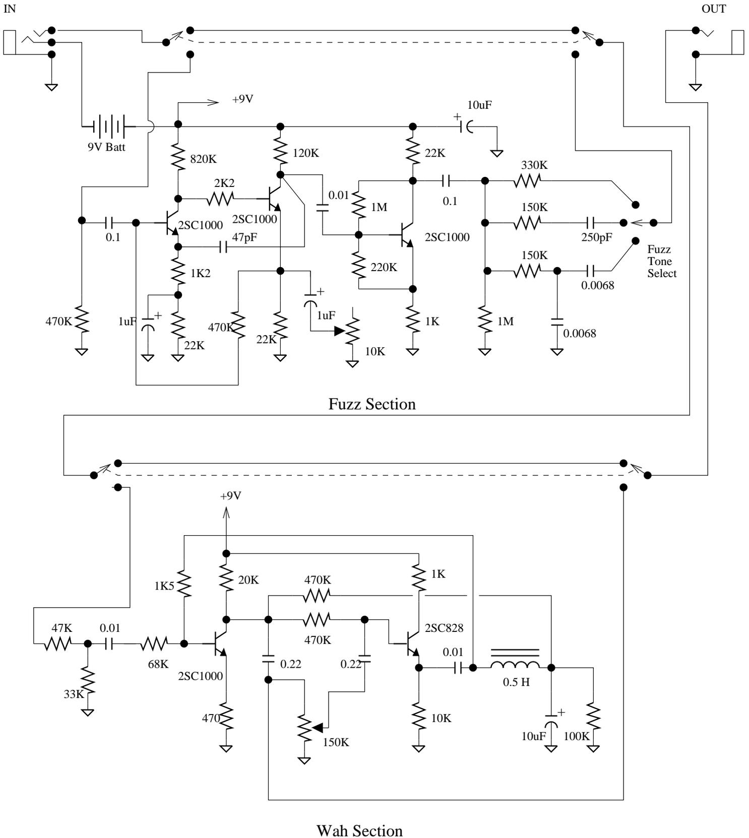
The Double Beat is another of those funky, funky Fuzz Wahs. The wah function is pretty standard, if a little quiet because of the resistive divider in front of the wah section cutting the signal down. The Fuzz section is pretty good, though. It has a good sound - no surprise as the first section is a lot like a Fuzz Face, but is followed up by yet another gain stage to distort even more. The three fuzz tone selections are **RADICALLY** different from each other.
