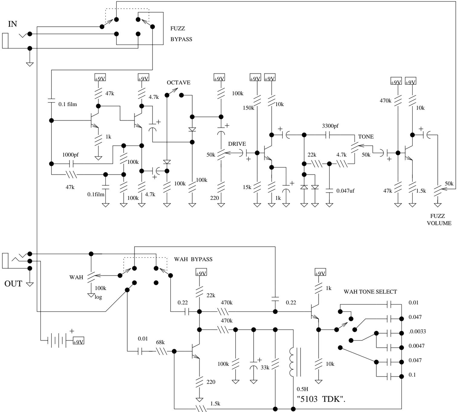
The Foxx Fuzz Wah includes a fuzz, an octave effect, a wah pedal, and in later versions a volume pedal all in the same box. The box, by the way, is covered in blue or red no-fucking stiff plastic fuzz. The wah has four different resonant frequencies selected by a rotary switch. The inductor should be relatively easy to find, as it looks to be a somewhat standard part. The volume pedal action is the default when wah is bypassed. Max volume is with the pedal all the way back, very odd.
