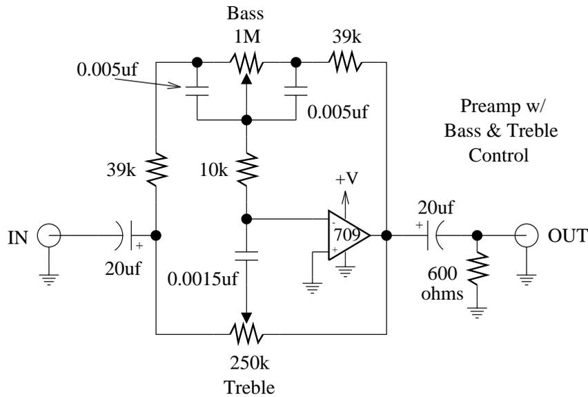
Both of these circuits provide some additional control over tone. They were originally intended for use with synth modules but could be easily incorporated into most any effects circuit.
