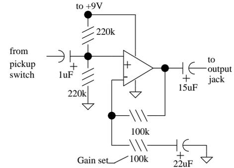
A preamp from a TL071 op amp. The gain set resistor lets you customize the gain. As shown, it is 2. Lowering the Gain Set resistor lets you raise the gain. You get distortion at high gains.
