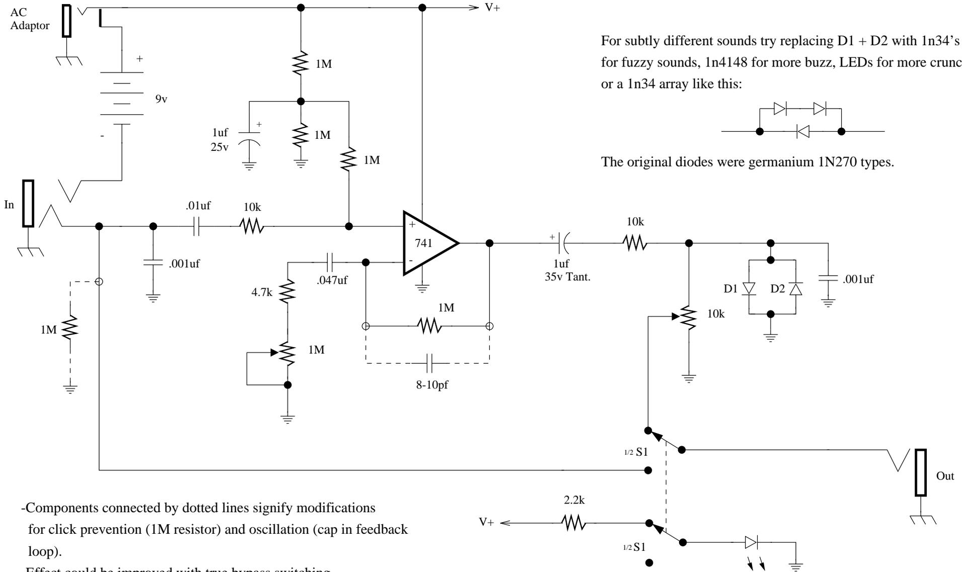
For subtly different sounds try replacing D1 + D2 with 1n34's for fuzzy sounds, 1n4148 for more buzz, LEDs for more crunch, or a 1n34 array like this:
