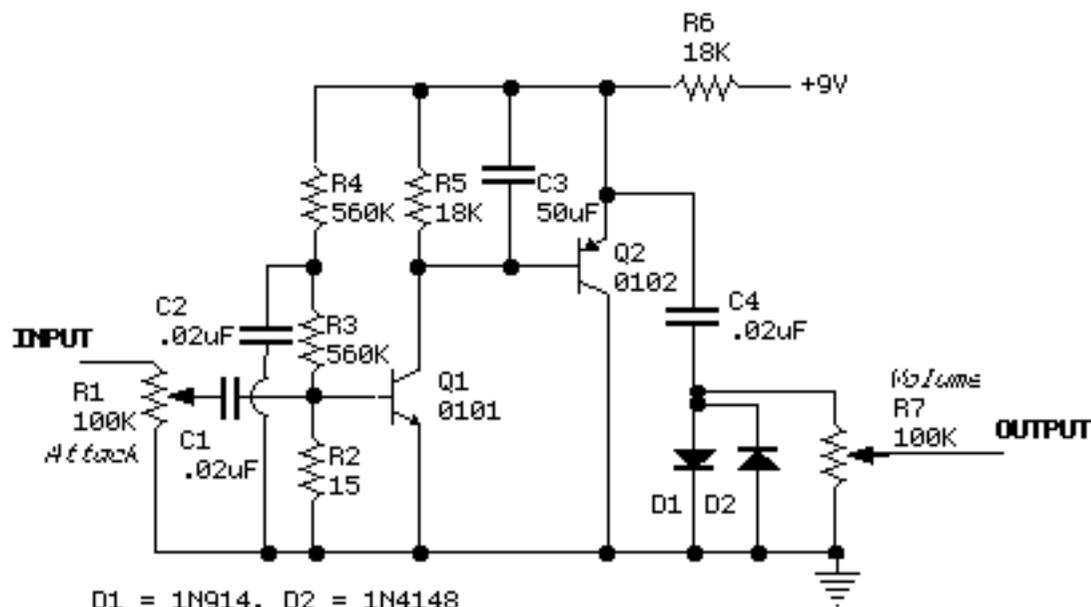
The Jordan BossTone as drawn in the factory schematic (minus switching circuit). The above circuit has been tested with the following modifications:
