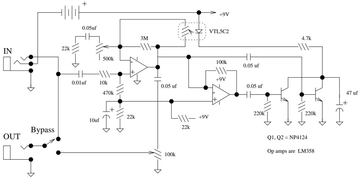
This is the original schematic, but it looks funny to me. I think that there should be a 100k resistor at the (-) input of the second opamp to make it a pure inverter. As it is, that stage would have a very large voltage gain, unbalancing what I think works as a full wave rectifier/current source for the LED in the compression feedback loop. I would expect that the proper circuit is as shown in the fragment below.
