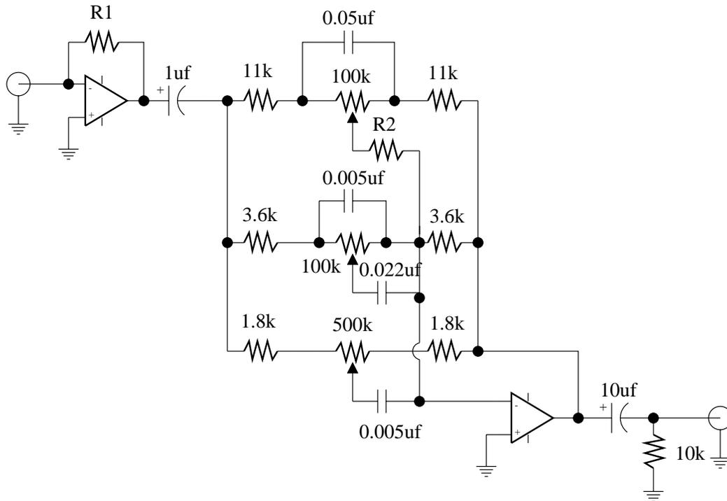
R1 is left up to the user depending on gain needs, R2 is unknown - experiment, the op-amps are not critical, any standard ones could be used. This circuit was originally intended for home audio use, but should be able to be hacked into an effect circuit with very minor modification.
