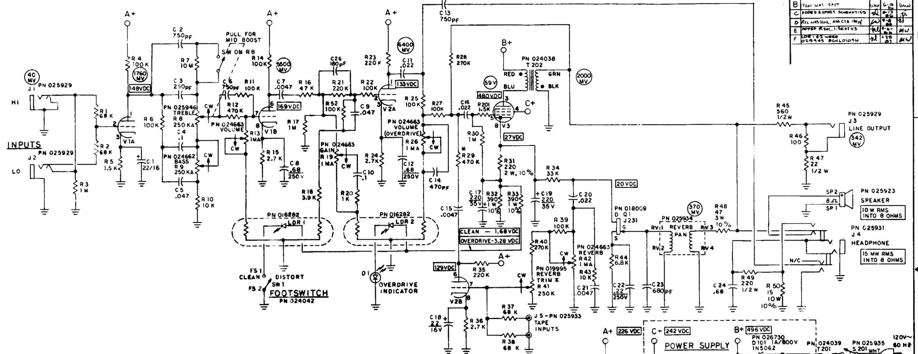
5. (MV) AC VOLTAGES DENOTE TYPICAL 1KHZ SIGNAL WITH AMP SET IN CLEAN MODE. ALL CONTROLS SET TO 12 O'CLOCK, REVERB AND MID BOOST OFF.
