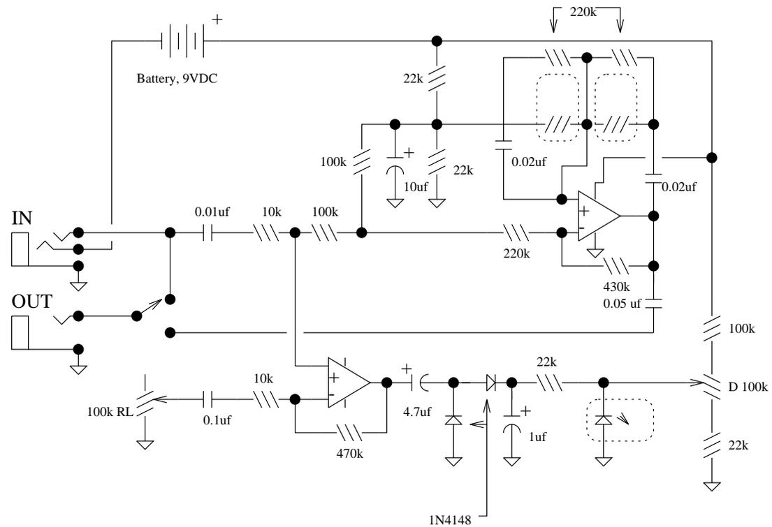
Opamps are each 1/2 of TL022 dual low power opamp. LED/LDR module is unknown, but is probably a Vactec VTL module with LED to center-tapped LDR.
