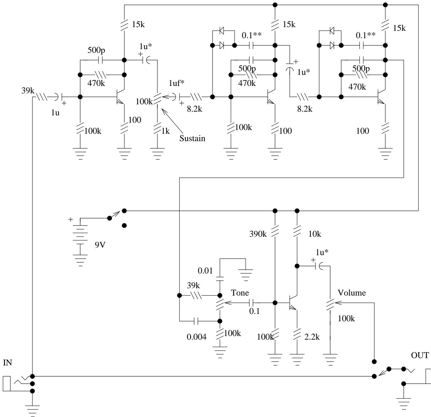
The EH Big Muff Pi would probably be improved by modern input-jack power switching and a DPDT bypass switch. This is the original schematic. The diode and transistor types are unknown. Probably any high gain NPN and 1N914s work. Coupling caps marked by a \* have been reported to sound better if changed to 0.1uF as have the \*\* marked ones if changed to 1.0uF. The original transistors were marked SPT 87-103, and the original diodes were marked 525GY or 523GY (hard to read).
