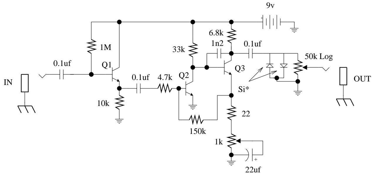
\*pretty much any silicon signal diode can be used here
